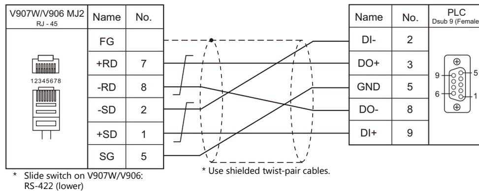
**Wiring diagram 5 - M4**
