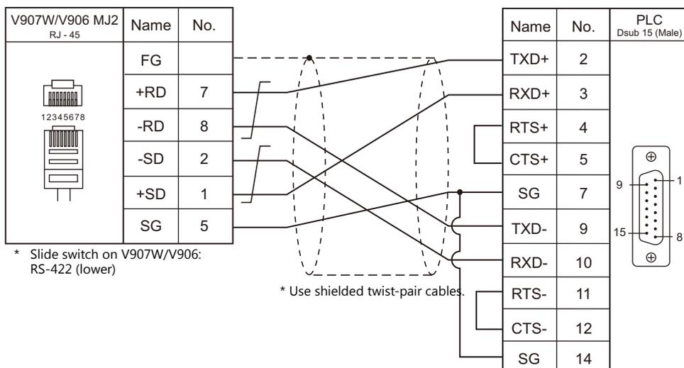
**Wiring diagram 3 - M4**
