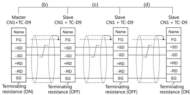
\* As a measure against noise, connect the frame ground terminal of each V9 series at one side only.
