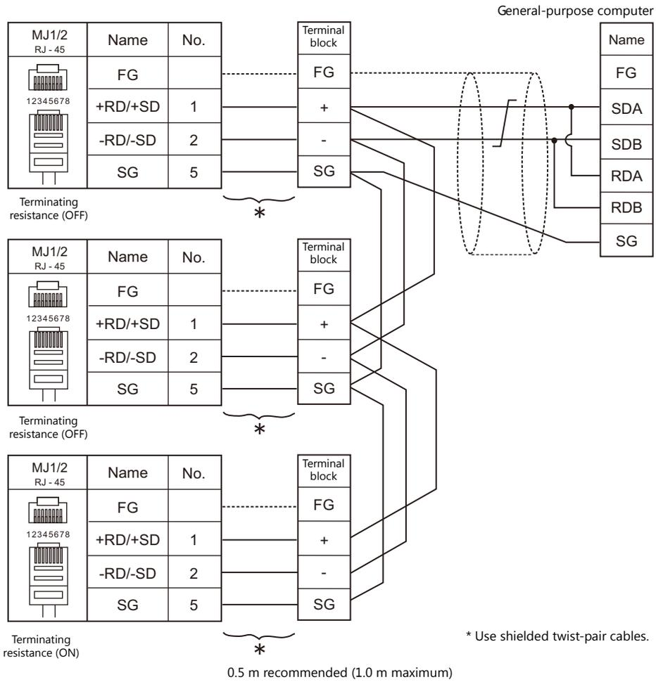
\* Set the slide switch for signal level selection to RS-232C/485 position (upper) when using the MJ2 port of V907W or V906. For details, refer to "1.2.2 MJ1/MJ2" (page 1-6).
