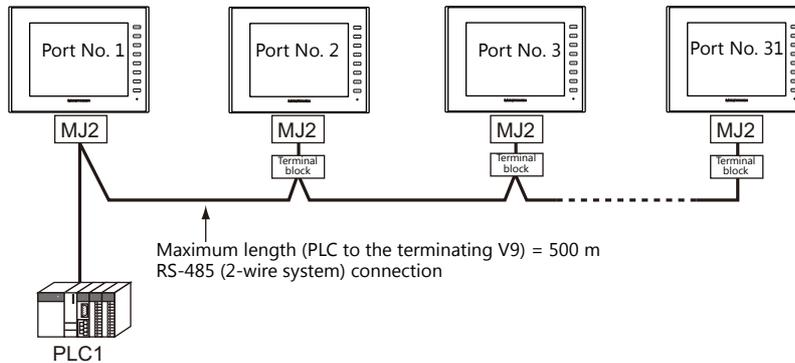
You can make settings for multi-link at the PLC1. Therefore, multi-link connection is not possible concurrently with a network connection that uses a "CUR-xx" communication interface unit. A physical port is selectable from CN1, MJ1, and MJ2.
