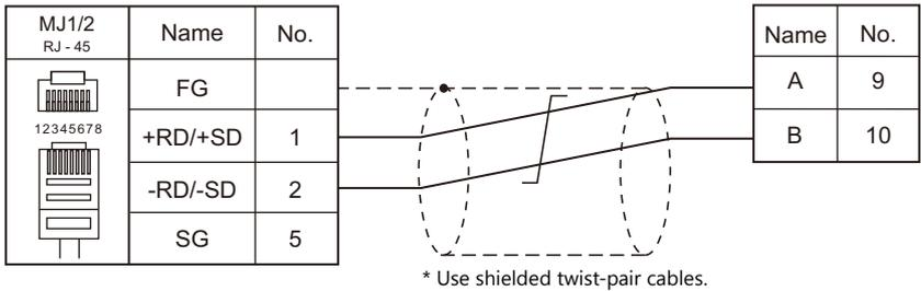
**Wiring diagram 6 - M4**
