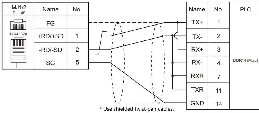
**Wiring diagram 6 - M4**
