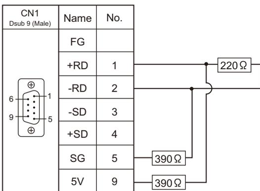
**Wiring diagram 3 - C4**
