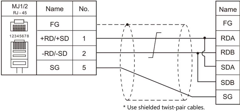
\* Set the slide switch for signal level selection to RS-232C/485 position (upper) when using the MJ2 port of V907W or V906. For details, refer to "1.2.2 MJ1/MJ2" (page 1-6).
