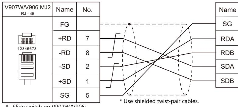
\* Slide switch on V907W/V906:
