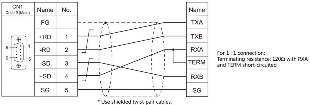
**Wiring diagram 2 - C4**
