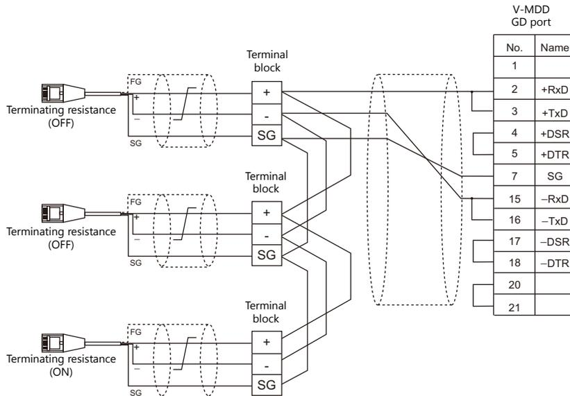
\* Set the slide switch for signal level selection to RS-232C/485 position (upper) when using the MJ2 port of V907W or V906.
