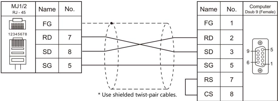
\* Set the slide switch for signal level selection to RS-232C/485 position (upper) when using the MJ2 port of V907W or V906. For details, refer to "1.2.2 MJ1/MJ2" (page 1-6).
