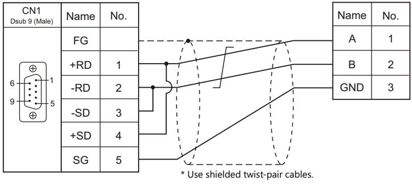
**Wiring diagram 4 - C4**
