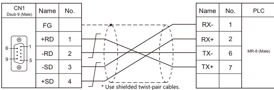
**Wiring diagram 4 - C4**
