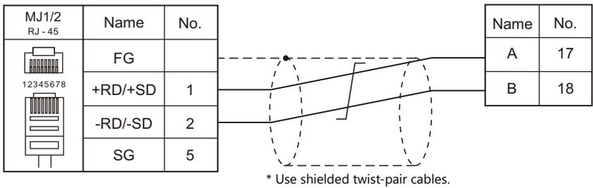
**Wiring diagram 5 - M4**
