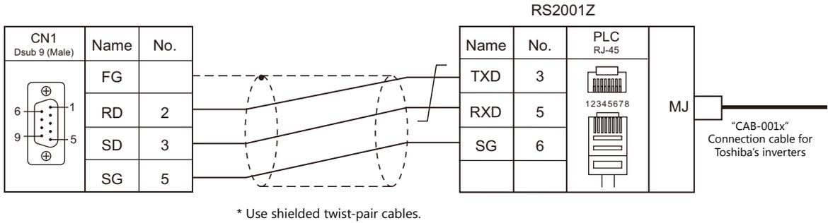
Wiring diagram 2 - C2
