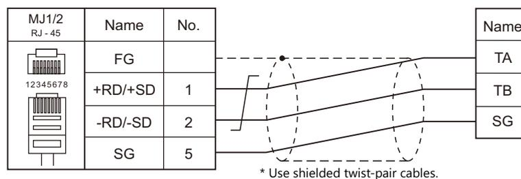
**Wiring diagram 2 - M4**
