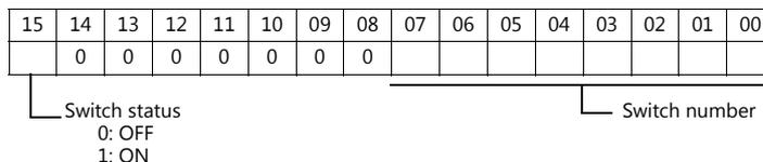
For the relationship between the switch output device memory and the switch number, see page 31-36.
