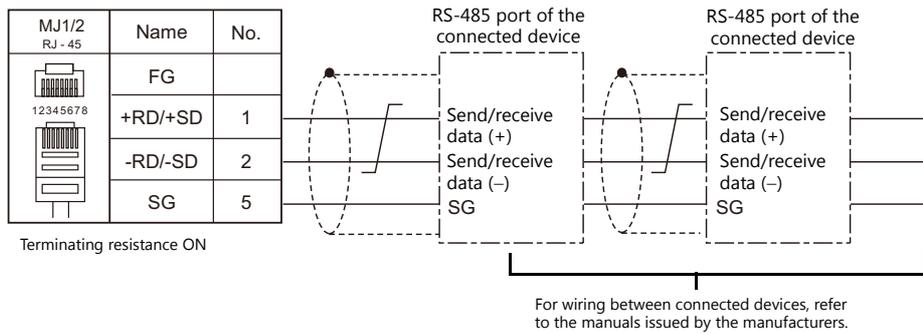
\* Set the slide switch for signal level selection to RS-232C/485 position (upper) when using the MJ2 port of V907W or V906.
