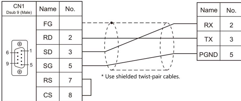
Wiring diagram 2 - C2
