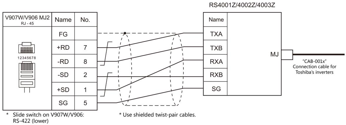
**Wiring diagram 5 - M4**
