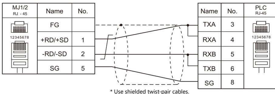
**Wiring diagram 3 - M4**
